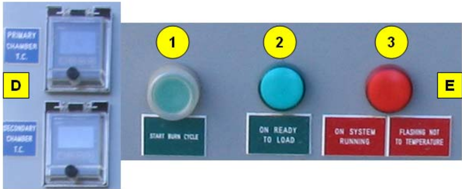
Figure 12 Sub-Section D: Temperature Controllers; E: PLC Indicating Lights and Control Button [CP6 to CP9 in Table 7]
