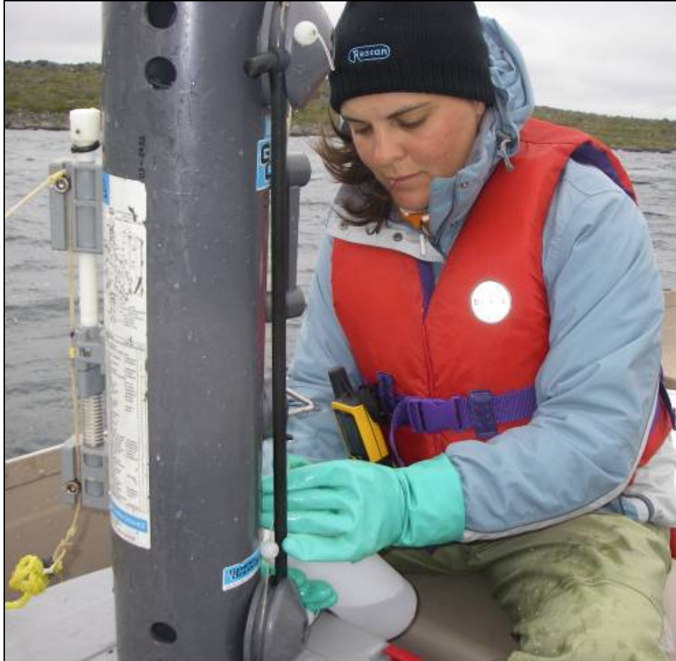
Plate 2.3-1. Lake water quality sampling with the use of a 5L GO-FLO.
