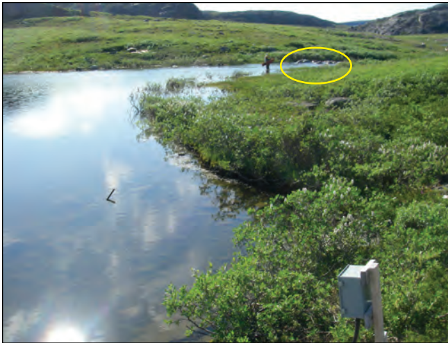
Left: Roberts Lake outflow looking downstream (northwest). The hydrometric station is on the foreground and was reestablished on June 21, 2011. The pressure transducer recorded water levels at 10 min intervals. The yellow circle indicates a riffle section in the channel that controls the rate of water flowing from the lake. Right: Close up view of the the control section (riffle). Farther downstream, on the background of the photograph, a fish fence can be observed. Photographs taken on July 22, 2011.
