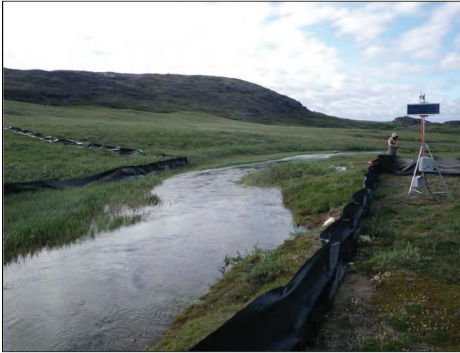
Left: Doris Outflow (TL-2) looking downstream (north). The hydrometric station is on the right bank. The pressure transducer and data logger recorded water levels at 10 minute intervals. The data were then sent to a web portal via satellite link and were available on a real-time basis. Right: Photograph of the same location now facing upstream (south). Note on the left bank the flood terrace with overgrown grasses where the channel overflows during high flow conditions. This causes the difference between the slopes of the rating relationship at low and high stage conditions. Photographs taken on July 24, 2011.
