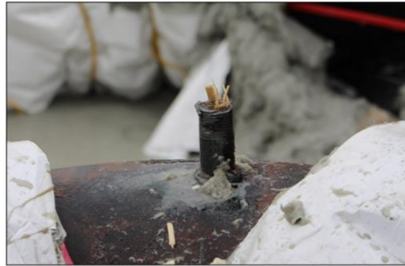
Worn threads on plugged inspection port prior to repair.
