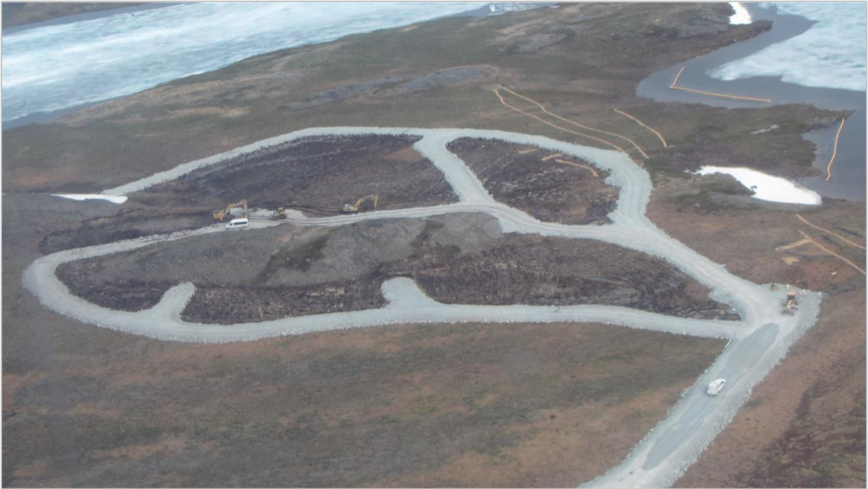
Figure 2. Overburden Stripping at Naartok East Crown Pillar Recovery Trench, June 2019
