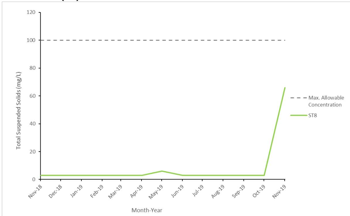
Figure 4. Total Suspended Solids Results Consistently Below Discharge Criteria for Wastewater Treatment Plant (ST8)
