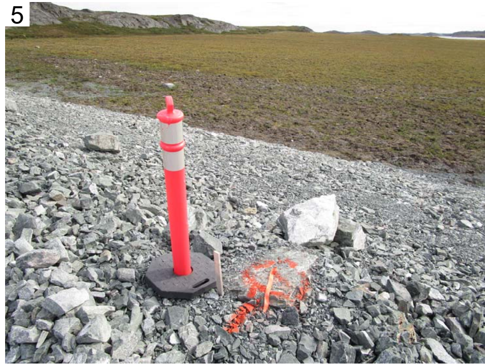
Photos: Photo 1: Aerial photo of the South Dam, looking east Photo 2: One of the data logger nodes on the upstream crest. Plywood casing is used to prevent animal damage. Photo 3: Close-up of the BeadedStream DL505 datalogger and solar panel units Photo 4: Photo along the crest showing the tailings discharges and monitoring instrumentation Photo 5: Example fixed settlement monitoring point along the crest Photo 6: One of the locations where a GTC has been repaired and will be further backfilled / covered (done post inspection)
