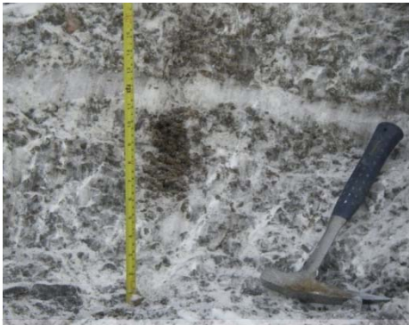
Ice lenses on exposed high wall
