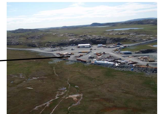
Light grey area in foreground is where stockpile crushed rock was stored. It has been removed without damaging tundra and drainage flows unimpeded.
