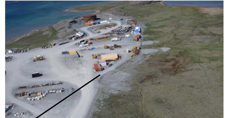
Northwest view across laydown area. Grey colour of tundra is where rock was removed. All drainage flows unhindered.
