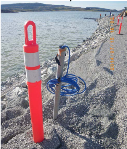
West side of jetty looking north, thermistor string SRK-JT-12 in foreground
