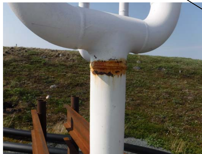
Rust observed at the weld between the evaporator pipe and the radiators.
