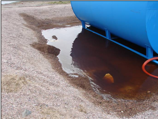
Photo # 24: Close up of contaminated soil and standing water within bermed area at airport
