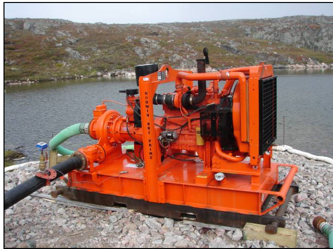
Photo # 1: Diesel Pump used to discharge water
