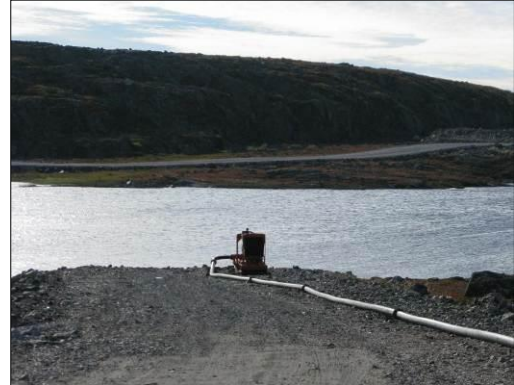
Photo 6: Water pump moving water from Cell B/C to PKCA for irrigation activity
