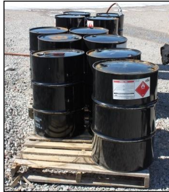
Photo 13: Barrels near bulk fuel tank farm stored without secondary containment.
