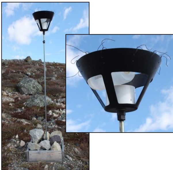
Photo 2: Dustfall monitoring station at West dam with overturned canister.
