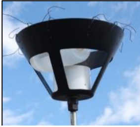
Photo 3: Dustfall monitoring station seen at the West dam as seen during the 2015 site visit
