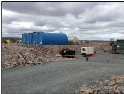
Photo 18: Incinerator (green stack) being used for burning remaining fuel and liquids (right in photo) and bulk fuel storage tanks (left in photo)
