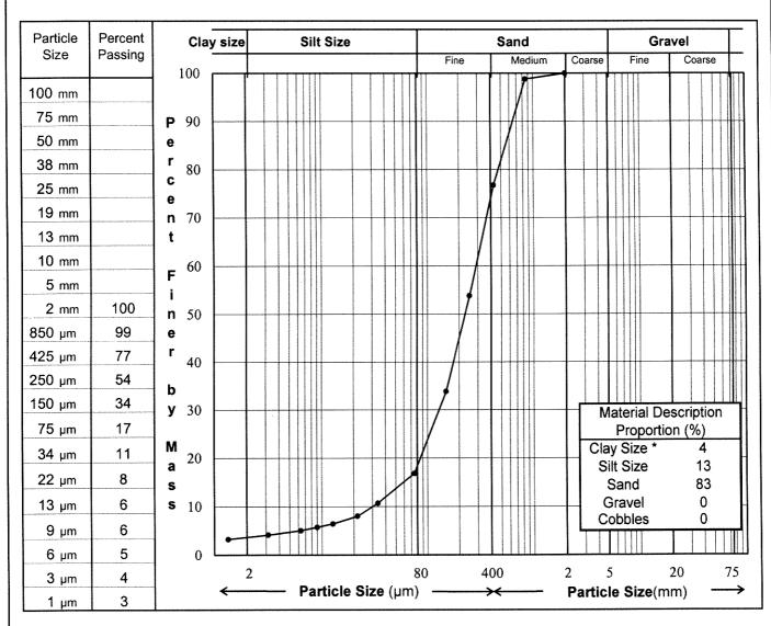
Remarks: \* The upper clay size of 2 µm is as per the Canadian Foundation Manual.
