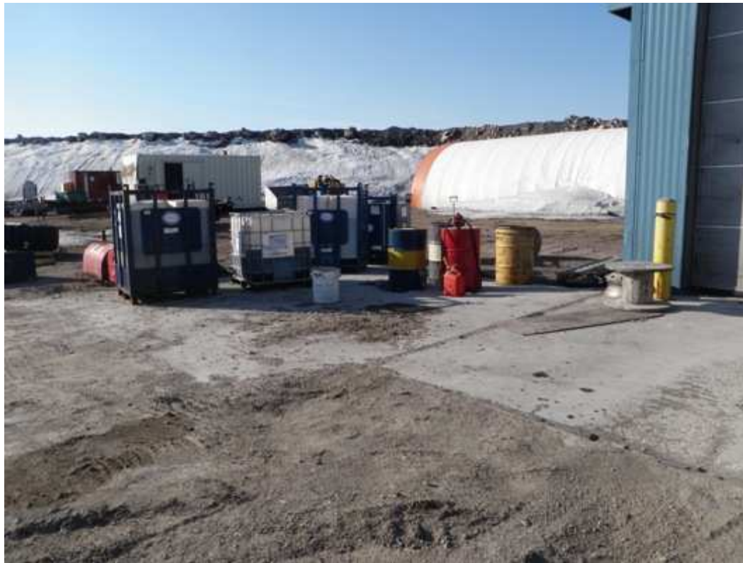
Photo 7 – Cubes and drums outside of the Truck Shop, no secondary containment
