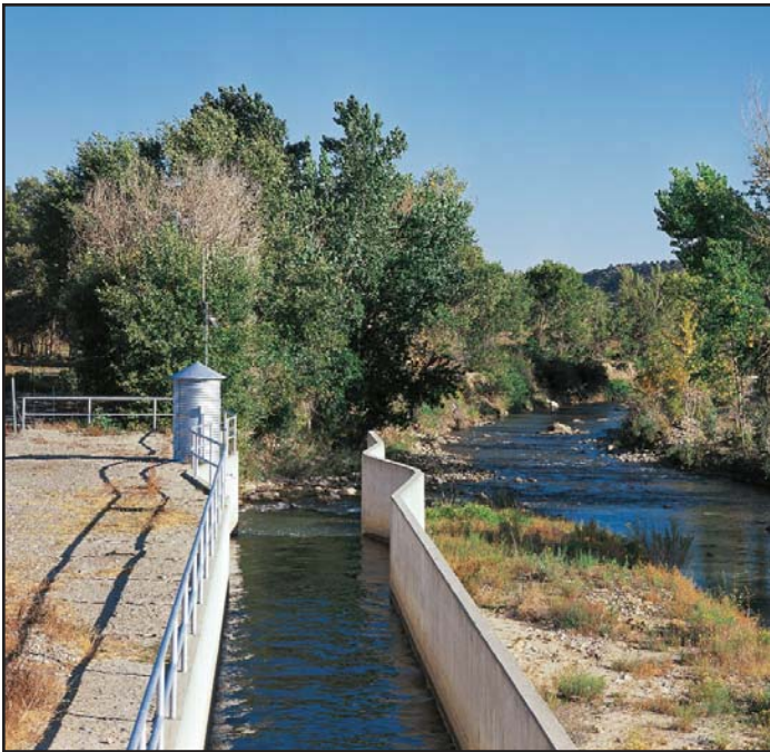
Datalogger measures water level using a shaft encoder, then calculates flow. The data are telemetered, via radio, to the water master for further processing, review, and archive. Stilling well at diversionary dam, Emery County, Utah.
