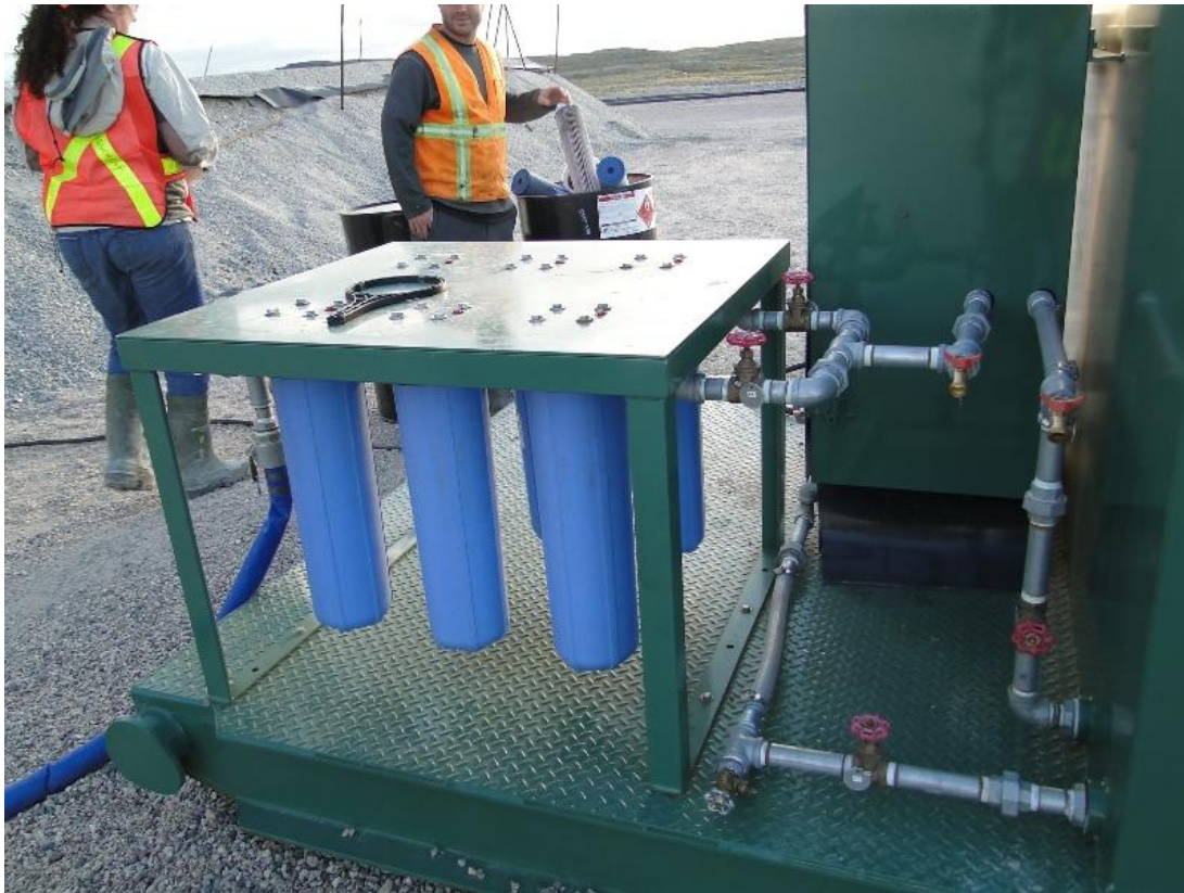
Figure 16. The Oztek uses a combination of filters and ozonation, and the only waste produced is a filter which can be incinerated.
