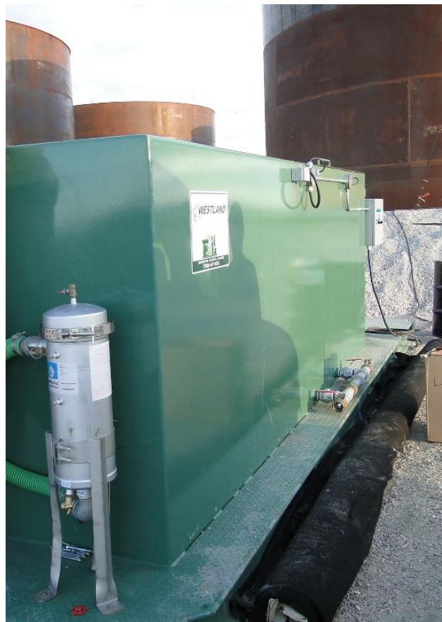
Figure 15. Shear has participated in the design of the Oztek Unit, a treatment unit for hydrocarbon-impacted water. They can now treat water on-site.
