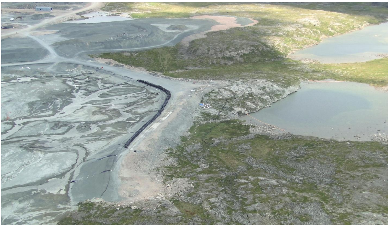
Figure 4. FPK blown towards SE pond. Note silt fences and berms in water to reduce transport of sediments.
