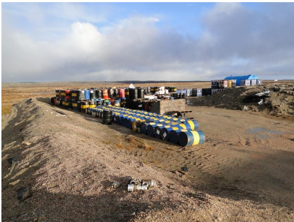
Figure 9. HWTa - barrels of old fuel should be upright to reduce likelihood of leaking.
