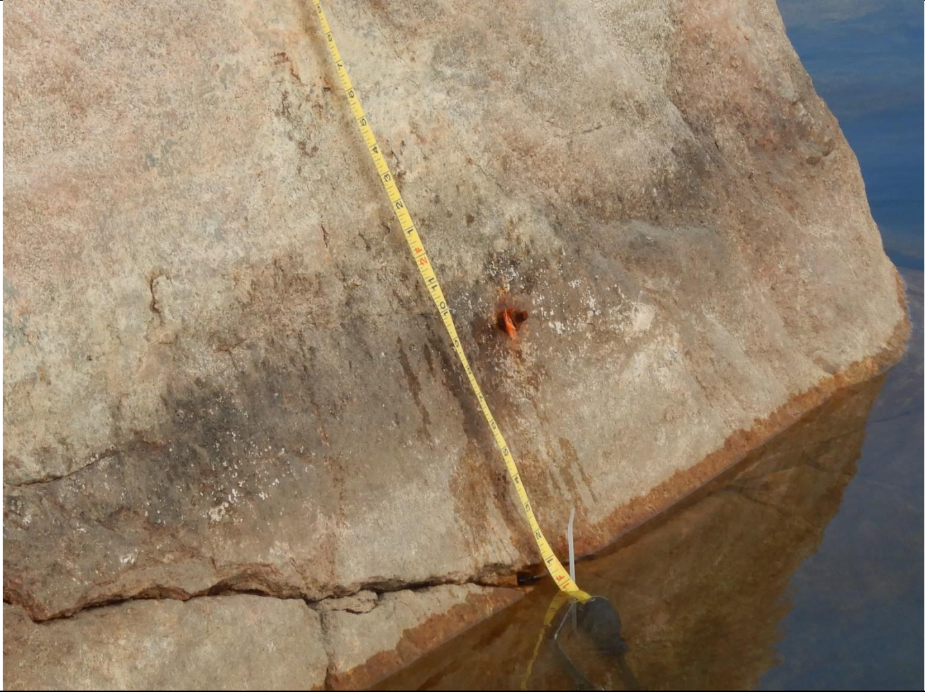
Description: Measurement from the Rock Bolt to the Water Line of Long Lake (PKCA Cell 2) showing at approximately 9 inches
