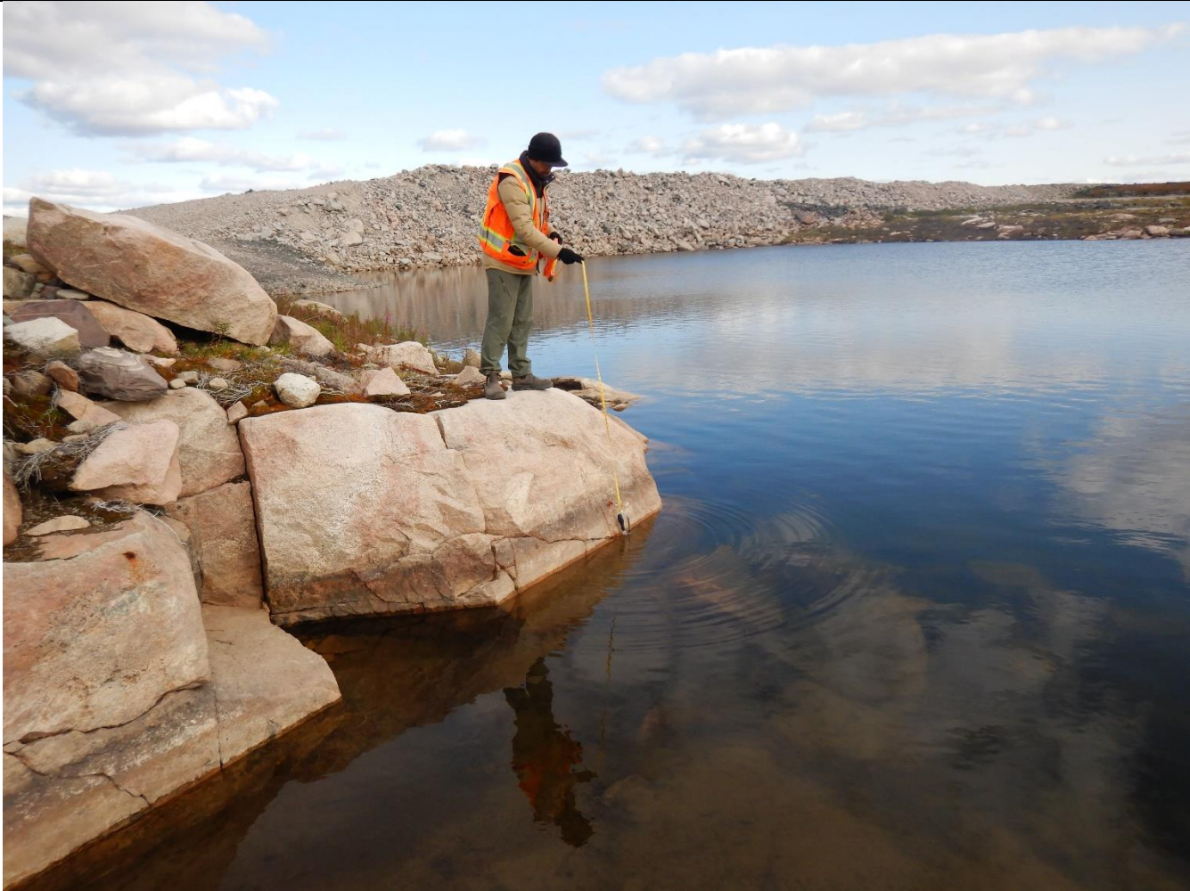
Description: Measuring the Level of Water to the Rock Bolt on the North Shore of Long Lake (PKCA Cell 2)
