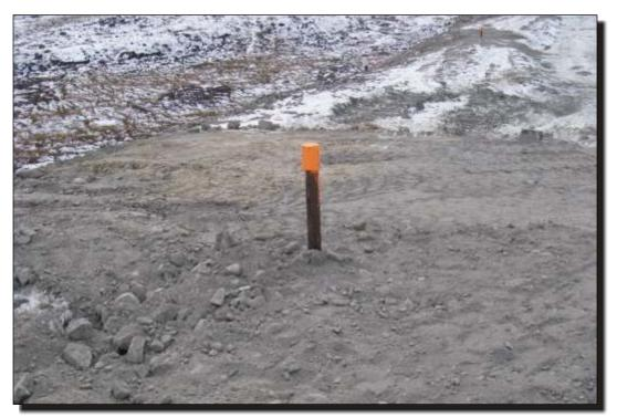
Photo 35 Southeast Dam Survey monitoring point.
