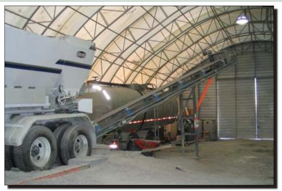
Photo 1 East Dam Reimer Truck Batch Plant.
