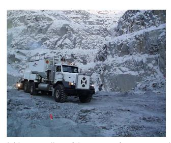
The bulk truck will mix the appropriate blend of diesel fuel with the AN prill and transfer this product to the pit for borehole loading of dry holes.
