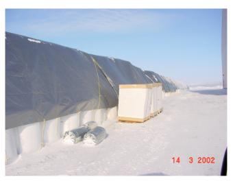
Ammonium Nitrate is packaged in a 1000 kg tote bag and shipped to site on flat deck trucks usually in 34 tonne loads. To minimize exposure to weather conditions the totes are tarped.
