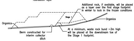
First stage of dump construction will consist of end dumping from dump crest towards the bund
