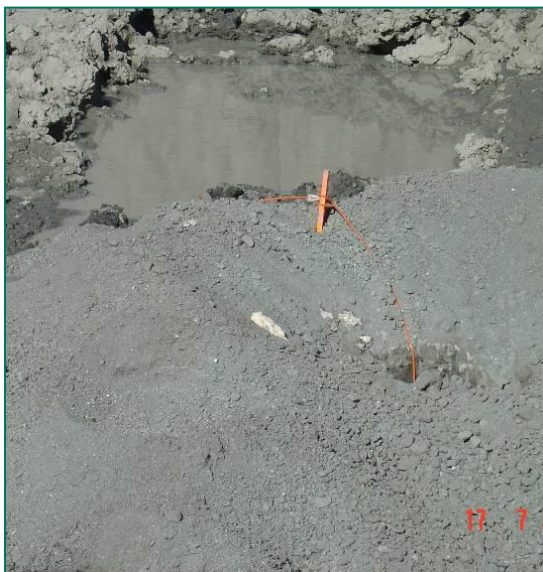
Photo 7.1: Emulsion spillage during transfer of loading hose from one pit hole to another
