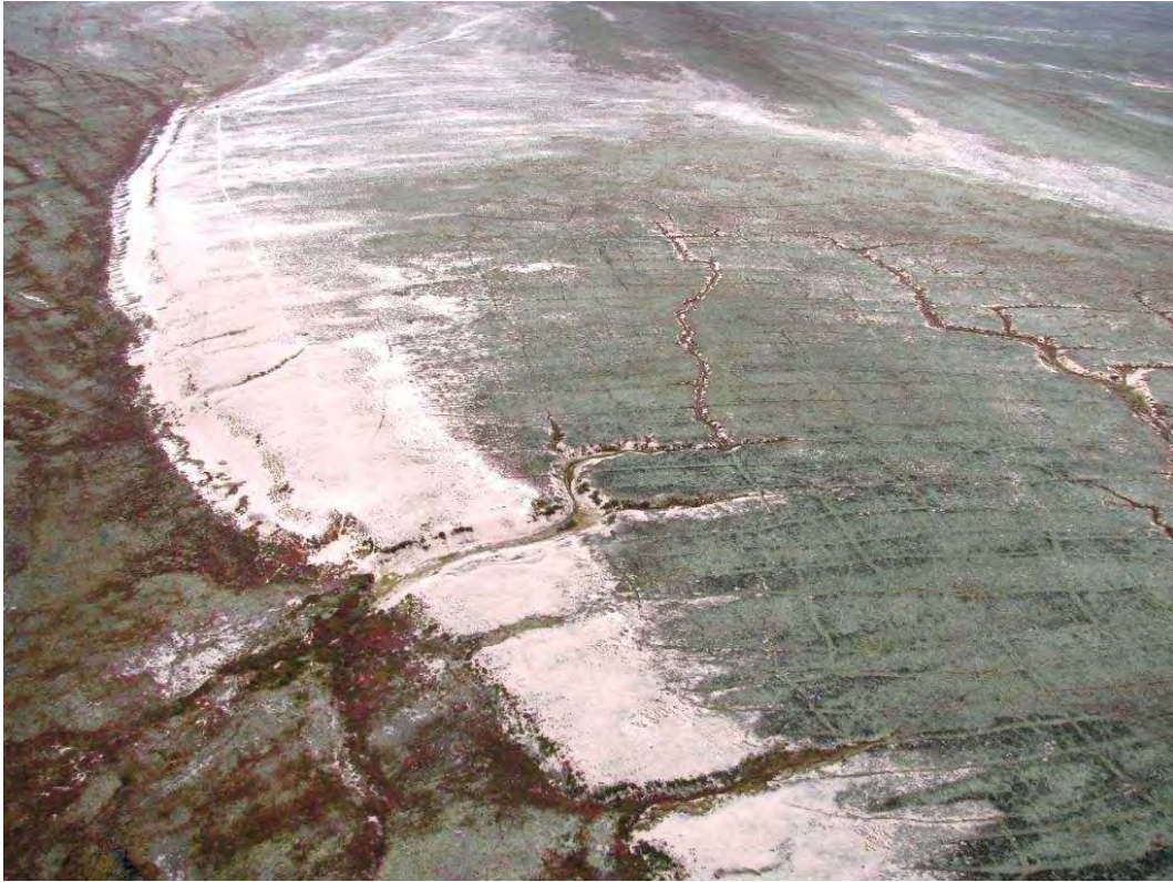
Marine Deposits near Baker Lake- (well-sorted sands with a percentage of gravel and cobbles)
