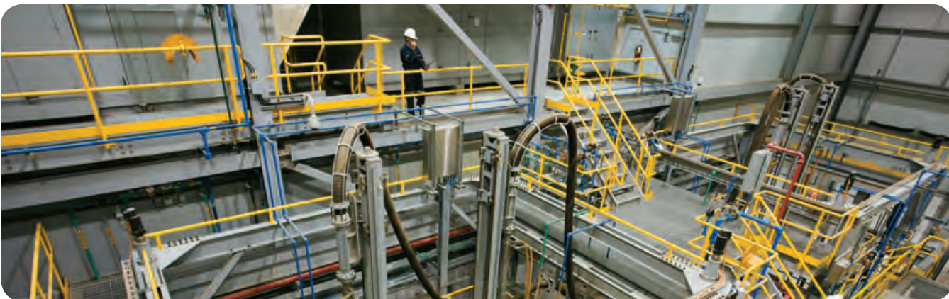
McClean Lake mill's new ore receiving circuit is built to accommodate high-grade ore from Cigar Lake.
