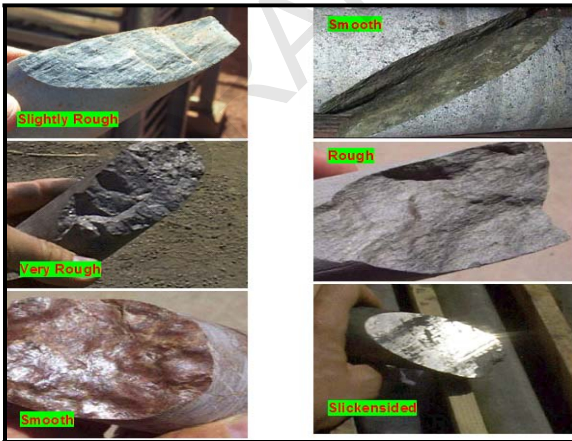
Figure 2.11c: Roughness of the joint walls
