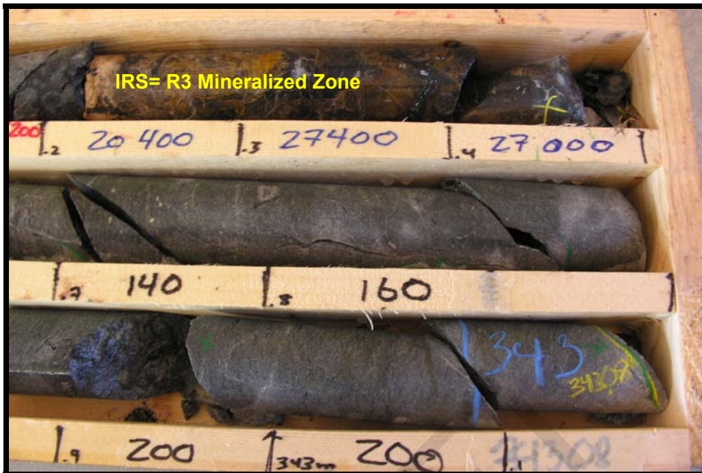
Figure 2.5: Estimation of Field Strength of drill core
