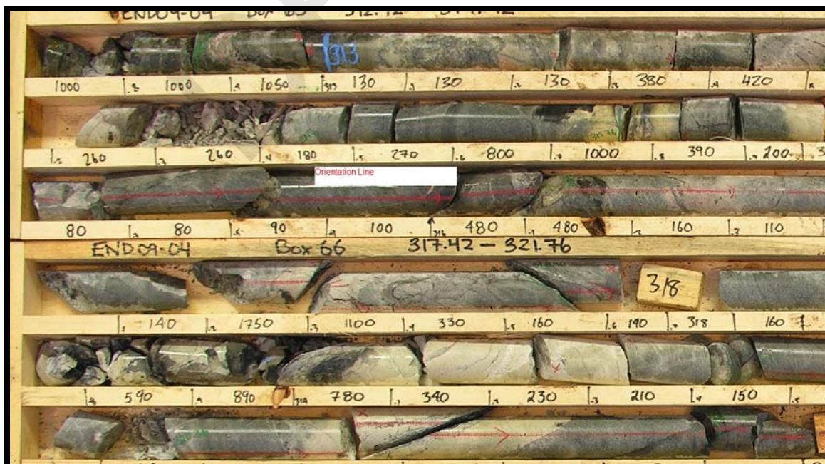
Figure 2.13: Core orientation line in drill core
