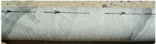
Orientation line on core. The barbs point 'down-hole' – that is away from the collar, even if the hole is directed upwards from underground.
