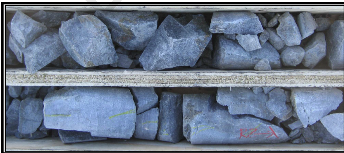
Figure 1.6: Illustration of Natural Rubble Zone (Broken Zone)
