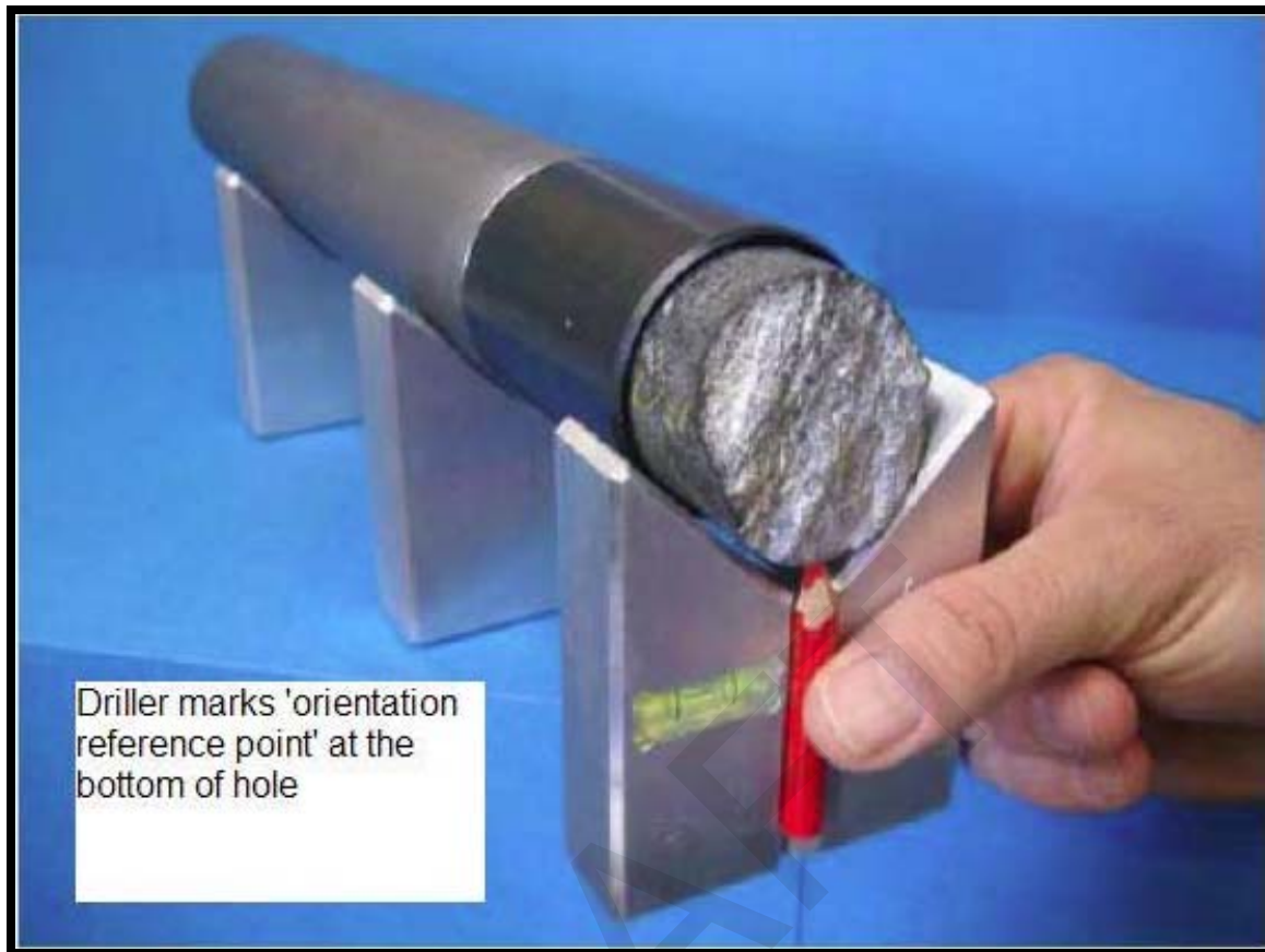
Figure 2.12: Demonstration of marking 'orientation reference point'
