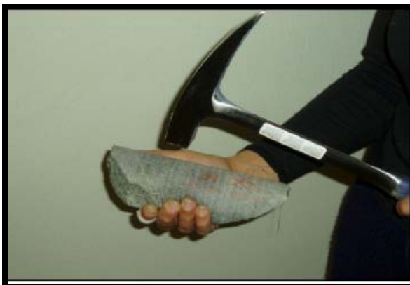
Figure 2.4: Rock pick test in drill core
