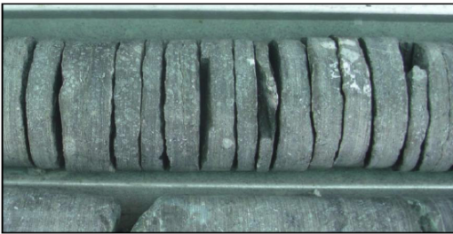
Figure 1.7: Illustration of mechanical breaks in drill core
