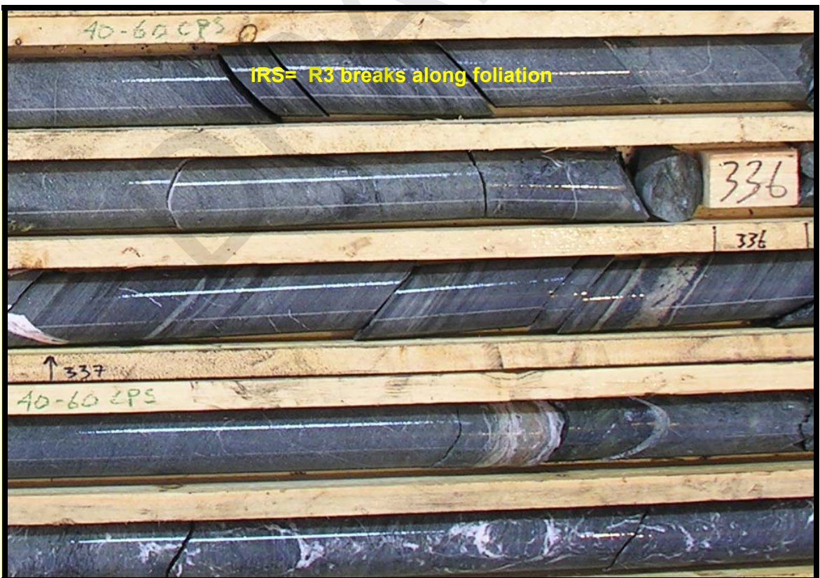
Figure 2.8: Estimation of Field Strength of drill core
