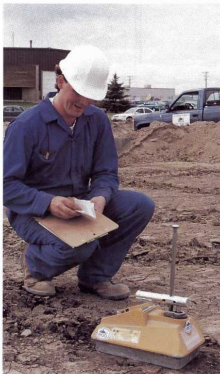
Field density determination using nuclear densometer
