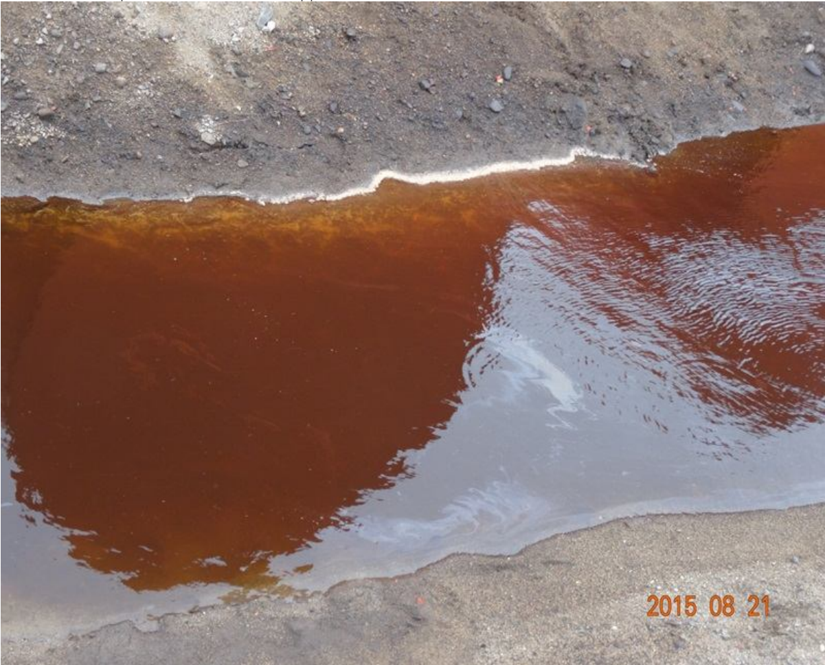
Figure 13 Satellite tank farm free product and emulsified oil on surface of water
