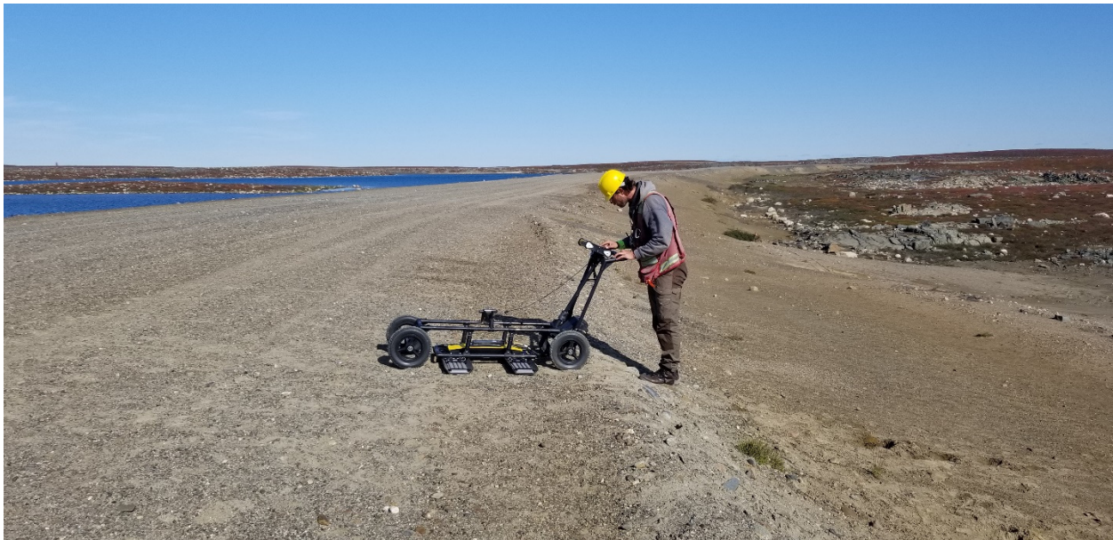
Figure 1. Operator performing the Ground Penetration Radar (GPR) cross profile on dam 4.
