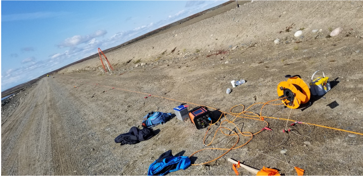
Figure 2. Electrical Resistivity Tomography setup on dam 3D.
