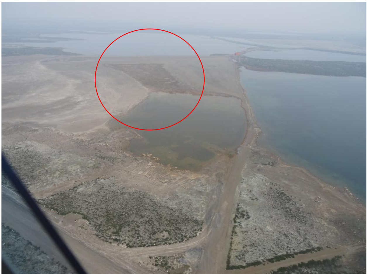
Figure 14. Dark patch shows the area of tailings still uncovered.
