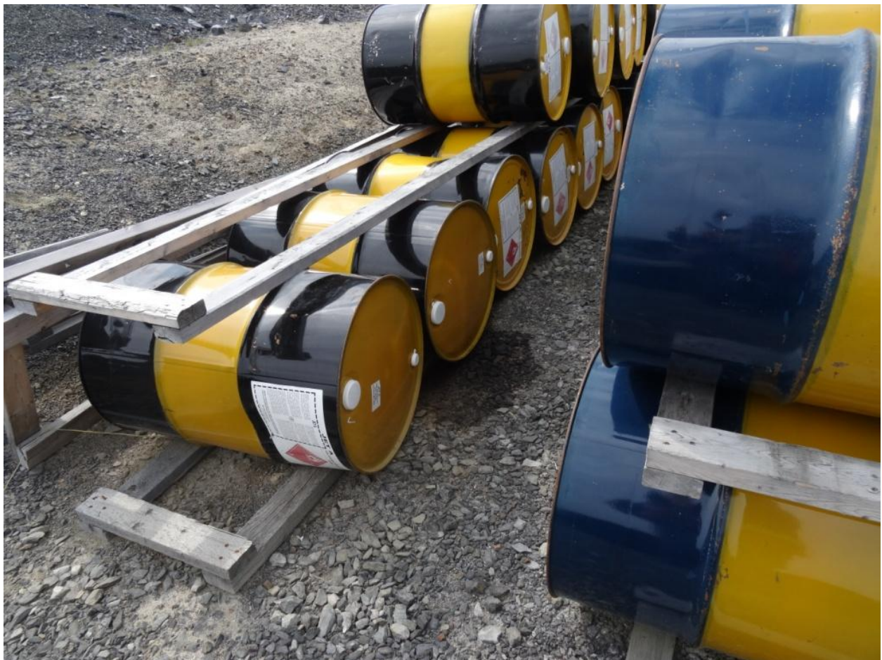
Figure 18. Barrel leaking in the 'Third Party' fuel berm.
