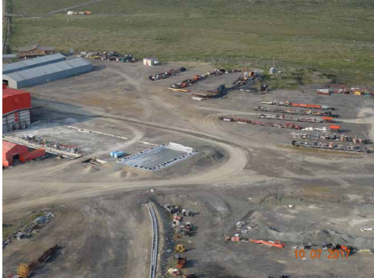
Description: View of landfarm from the air. Awaiting NWB approval and final fill prior to use. Water present in the liner at this time is non-contact water, accumulated from precipitation.
