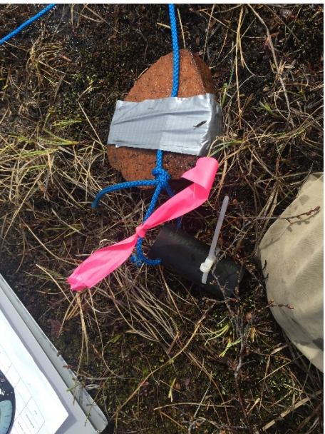
Photograph 1: Temperature loggers installed within a protective casing and anchored on a rock, June 2016
