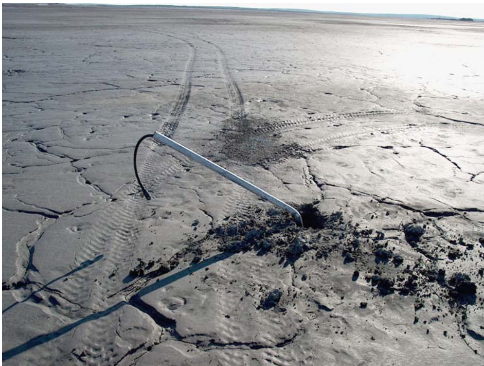
Photo 11 – Thermistor installed upstream of Dam 6 (Cell 3). Also attacked by a bear, but still useable.
