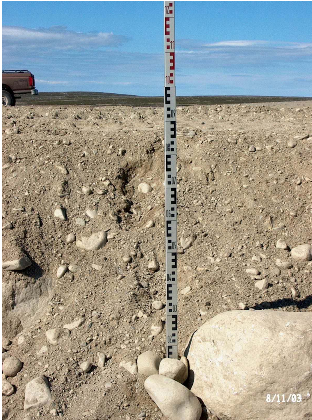
Photo 7 - Typical depth of esker cover on Cell 3A and 3B.
