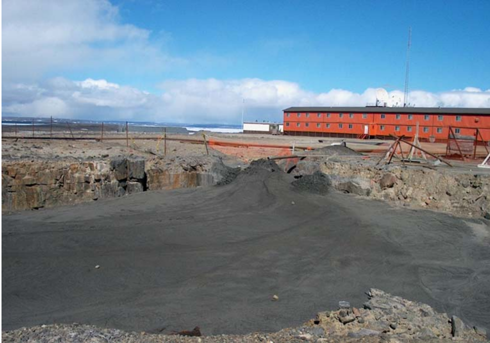
Photo 1 - Paste backfill being poured into Centre Zone crown pillar stope. View to east.
