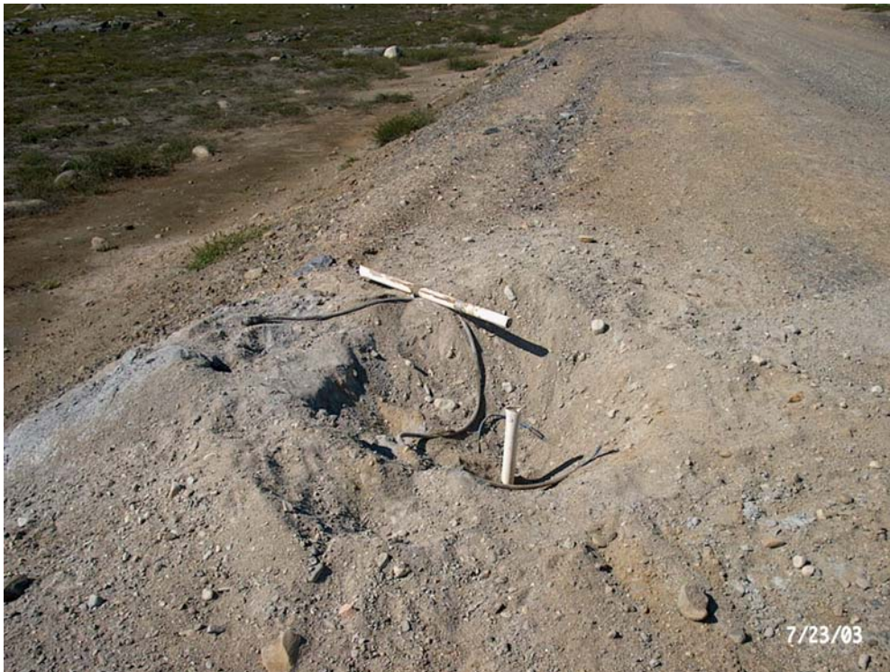
Photo 10 - Thermistor installed in Dam 6, destroyed by bear.
