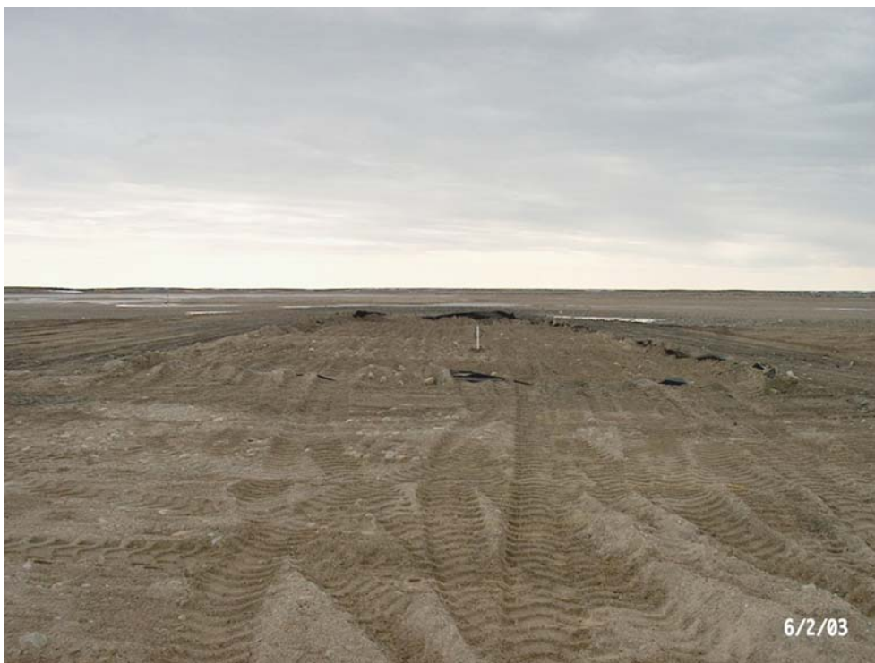
Photo 9 – Cell 1 test pad after liner installation and grooming. Note thermistor (white pipe) in centre of test pad.
