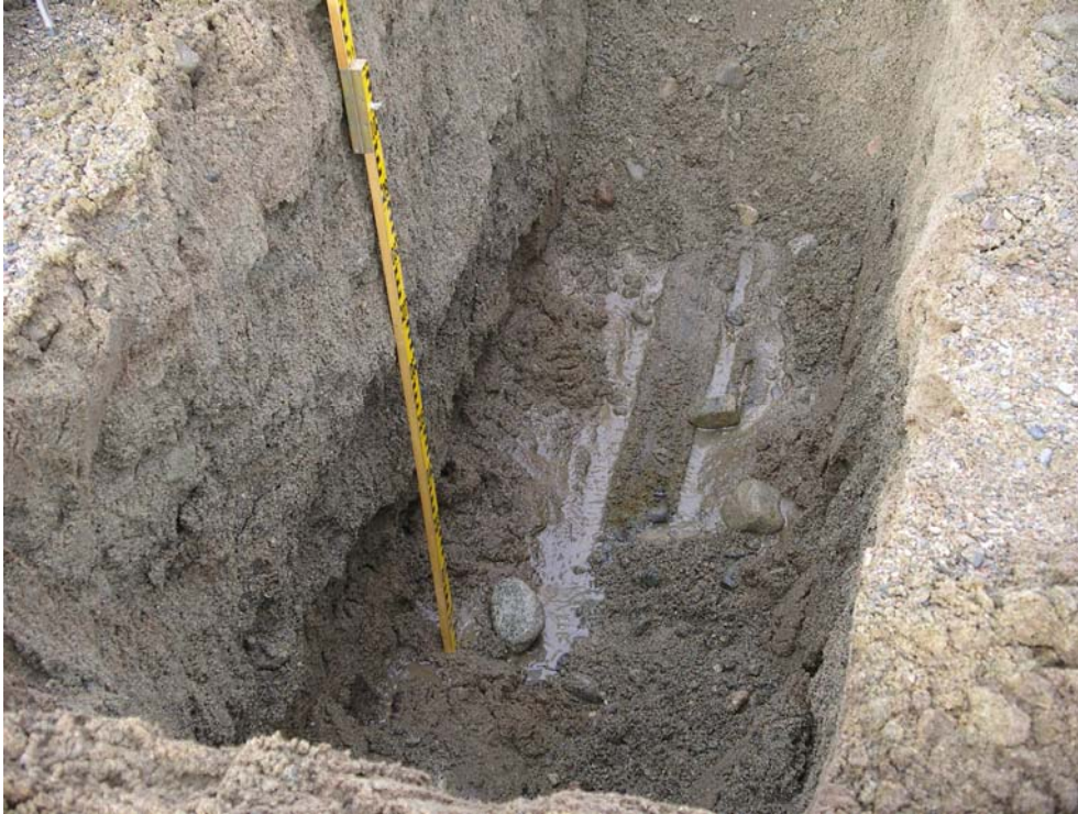
Photo 9 – Test Pit 1A-1, through the esker cover in Cell 1A. Cover was placed in 1988. Note moisture at tails interface.
