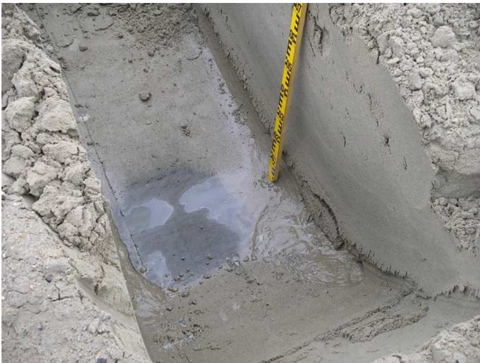
Photo 10 - Test pit 2-2, through esker cover in Cell 2. Cover was placed 2 months earlier. Note moisture at tails interface.
