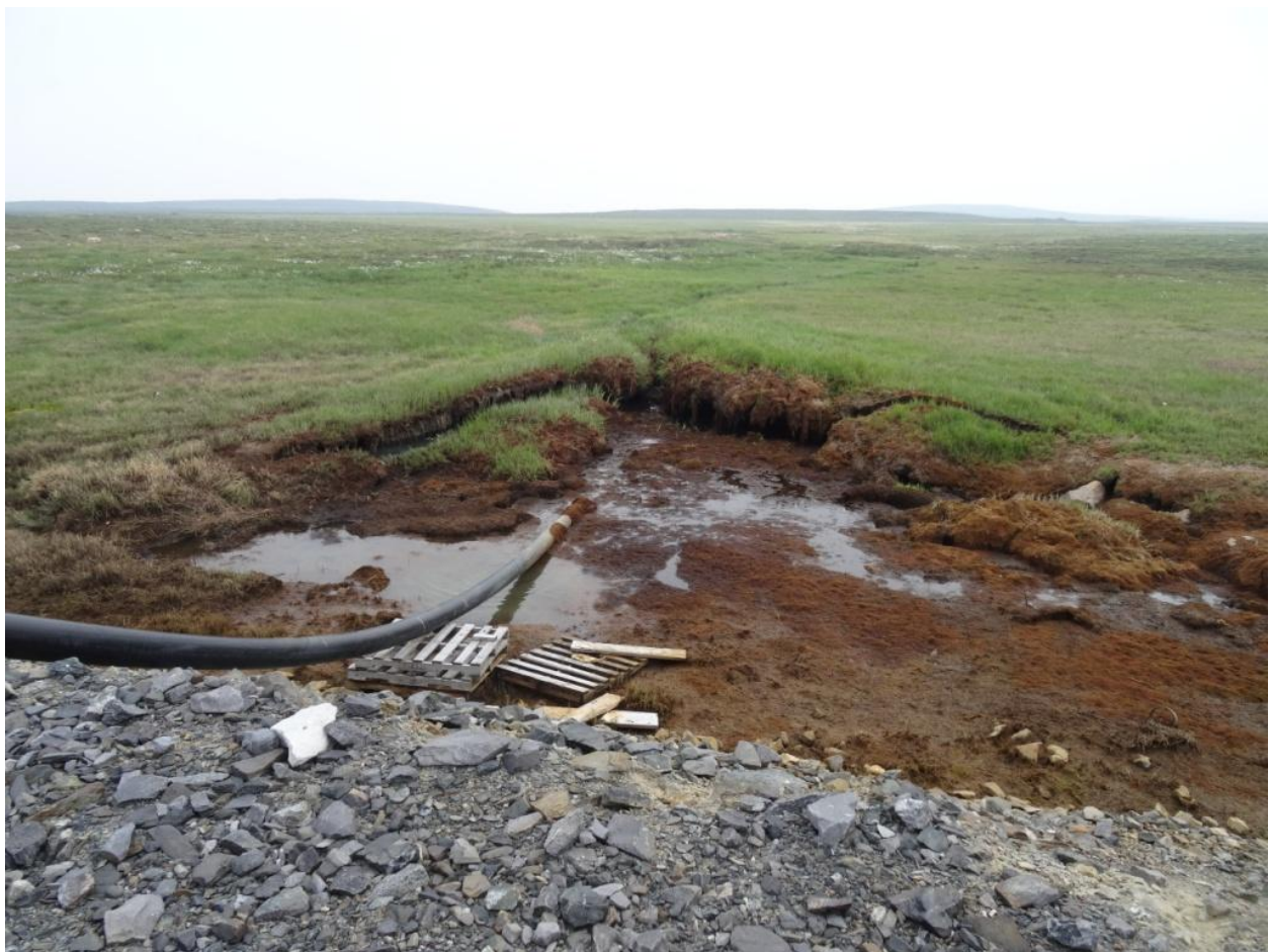
Figure 11. Permafrost degradation noted at discharge from LSL.
