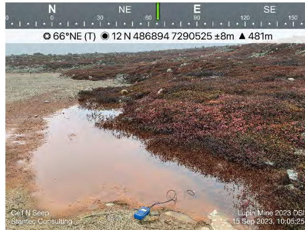
Photo 67: Sample ID Cell N-Seep 1 was collected from this waterbody situated against the native tundra at the Cell N cover tie-in point. Field readings indicated a pH of 3.48 at this location.
