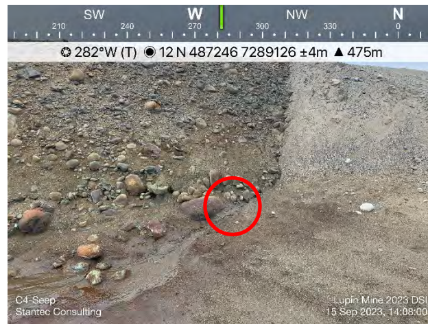
Photo 70: Close-up view of the point of outflow (outlined in red) for the acidic seep at the NW corner of Cell 4. Water was actively flowing from this acidic source at the time of sample collection.
