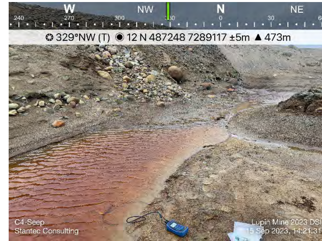
Photo 71: A water quality sample was collected just downstream of the point of outflow for the Cell 4 acidic seep. Field readings indicated a pH of 2.95 at this location.
