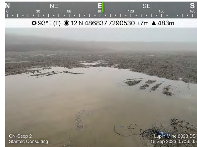
Photo 68: Sample ID CN-Seep 2 was collected from this waterbody situated on the Cell N cover. Field readings indicated a pH of 4.79 at this location.
