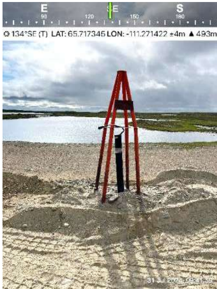
Photo 31: Thermistor D4-3. The thermistor was repaired on July 26, 2024.
