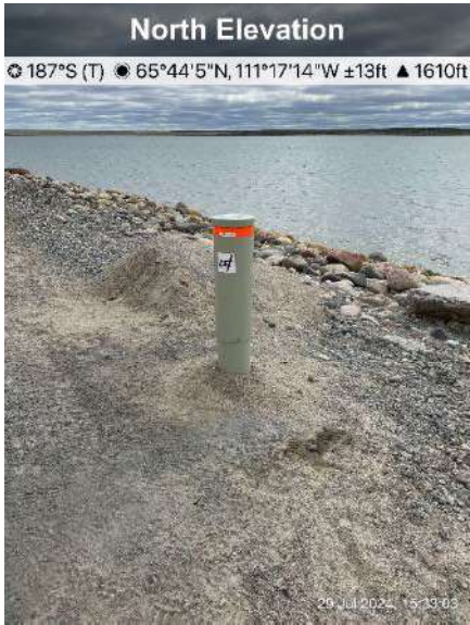
Photo 57: Thermistor DN-1-2024, installed in N Dam on July 21, 2024.
