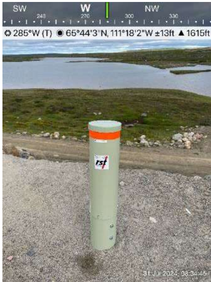
Photo 18: Thermistor D2-4-2024, installed on July 21, 2024, on Dam 2.
