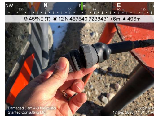
Photo 18: View of the damaged thermistor
