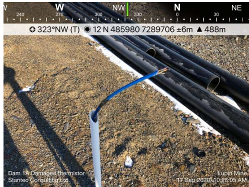
Photo 3b: View of the damaged thermistor.
