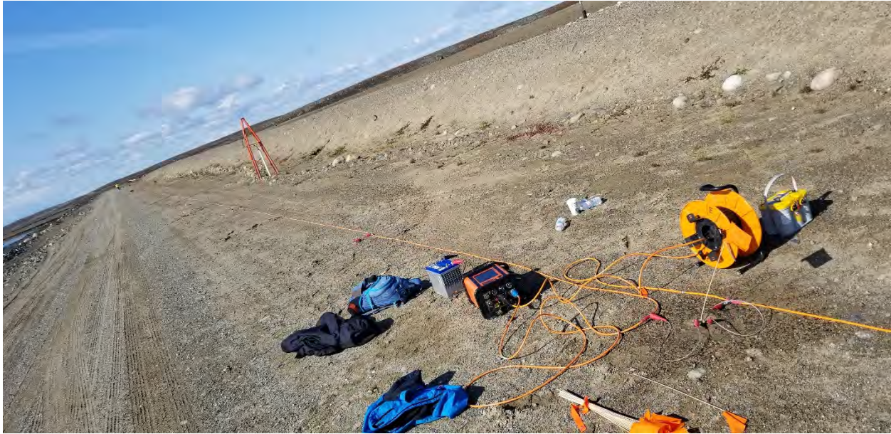
Figure 2. Electrical Resistivity Tomography setup on dam 3D.
