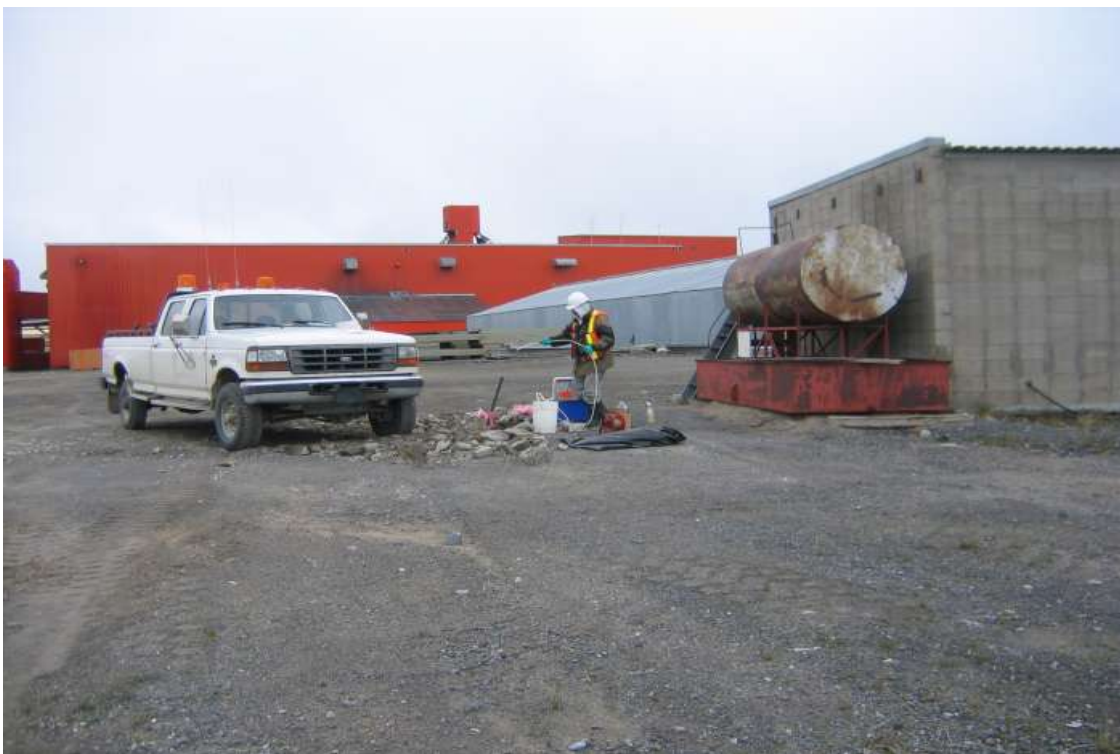
Photograph 38: View to east showing water sampling at monitoring well 05-15 adjacent to the incinerator, July 2005 (APEC 8b).
