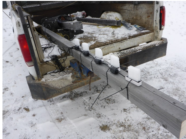
Photo 38: A string of 5 sensors mount on post, spaced 20cm apart waiting in preparation for installation.
