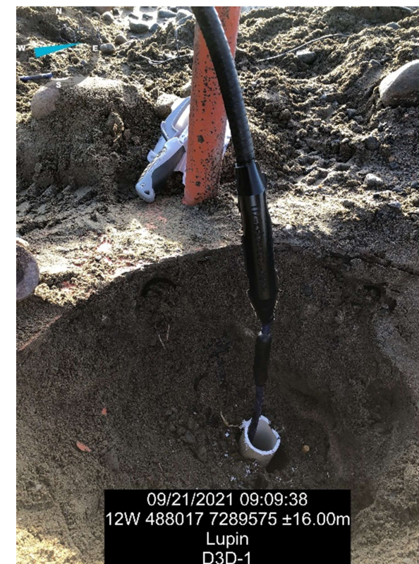
Photo 30: Finalized repair of the D3D thermistor.
