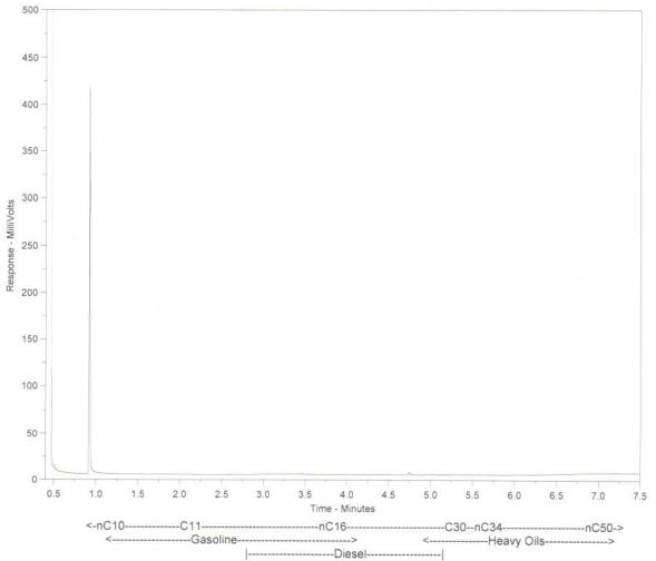
The Canada Wide Standard Hydrocarbon Distribution Report is intended to assist you in characterizing hydrocarbon products that may be present in your sample. The scale at the bottom of the chromatogram indicates the approximate retention times of common petroleum products as well as a number of specified n-alkane hydrocarbon marker compounds. Comparison of this report with those of reference standards may also assist in characterizing hydrocarbons present in the sample.
