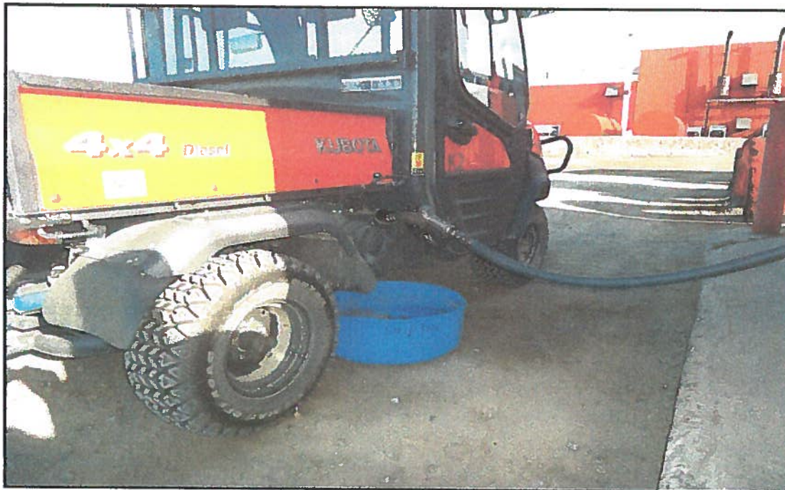
Photo 4: Lupin Mine Re-fuelling Station showing the use of a drip pan (July 23, 2012)
