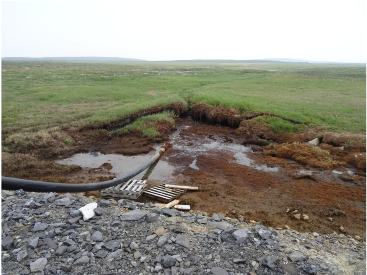
Figure 11. Permafrost degradation noted at discharge from LSL.
