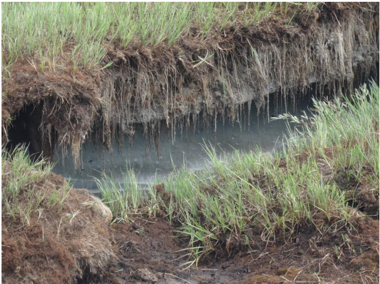
Figure 12. Ice lens forming at discharge from LSL. Closeup of Figure 11.
