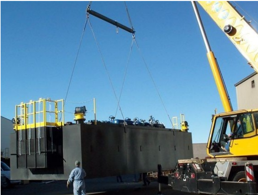
Barge being loaded for shipment – Note intake screens on end of hull
