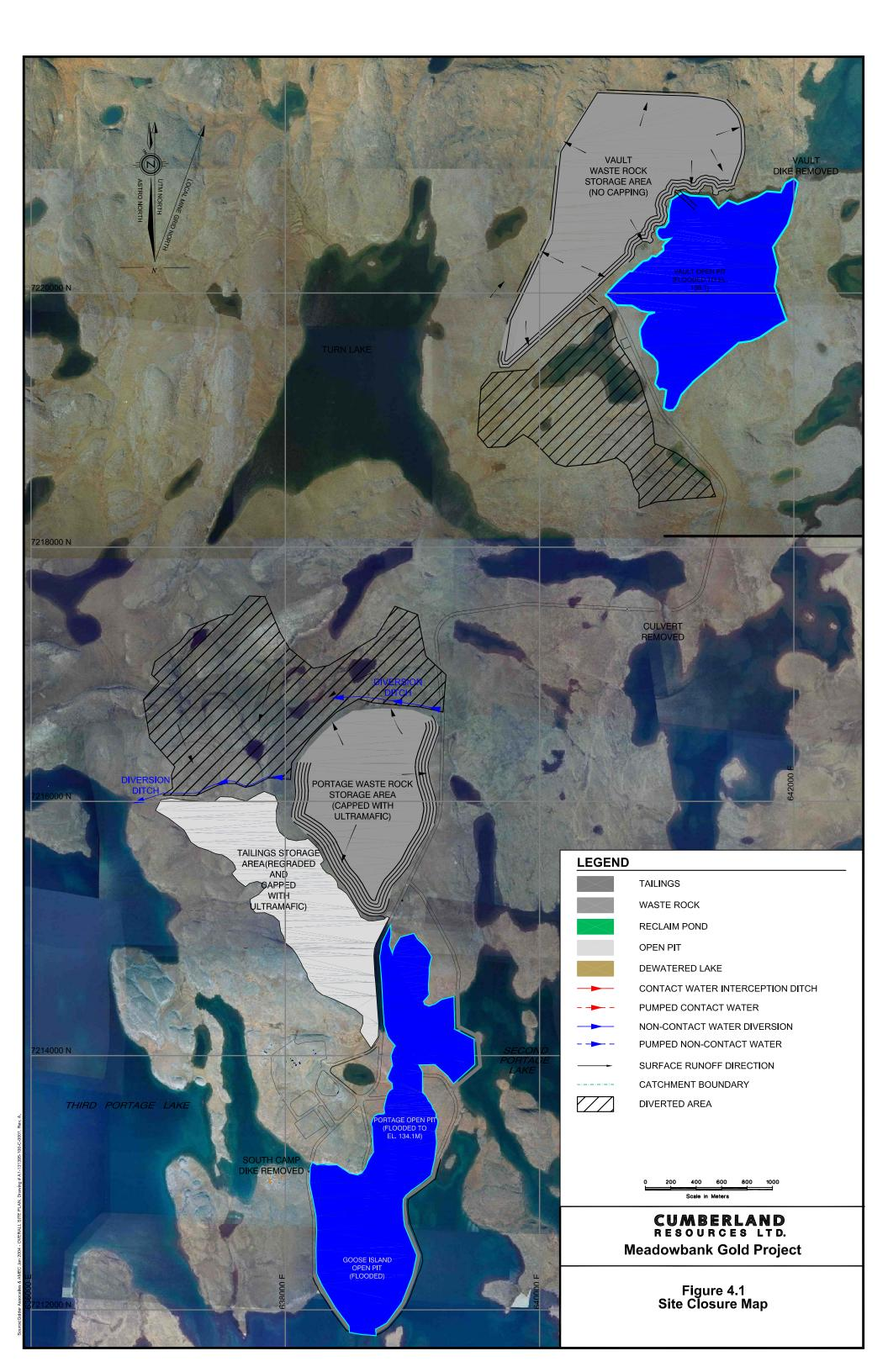
inflows from the lake watershed and will discharge south through the breached Bay Zone and Goose Island dewatering dikes into Third Portage Lake. Goose Island will be completely flooded. The East dike will be preserved to maintain a water level differential of about 1 m between Second and Third Portage lakes.
