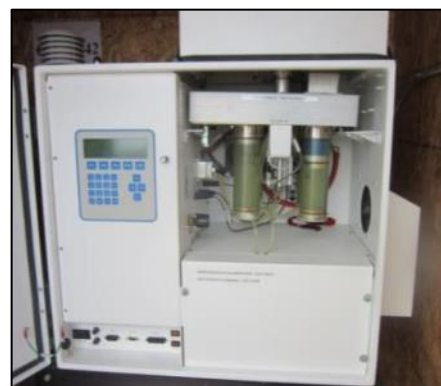
Photo 49: Station for the sampling of total suspended solids in air.
