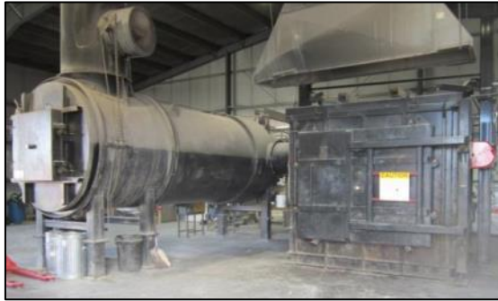
Photo 50: Meadowbank dual chamber incinerator, with secondary chamber on the left side.
